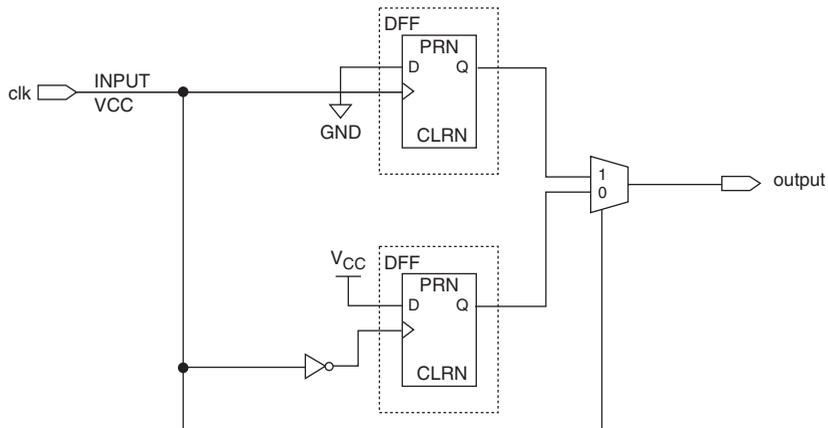
When an FPGA PLL generates the internal clock, the PLL output clocks the IOE block. As the PLL only monitors the positive edge of the reference clock input and internally re-creates the output clock signal, any DCD present on the reference clock is filtered out. Therefore, the DCD for a DDIO output with PLL in the clock path is better than the DCD for a DDIO output without PLL in the clock path.
