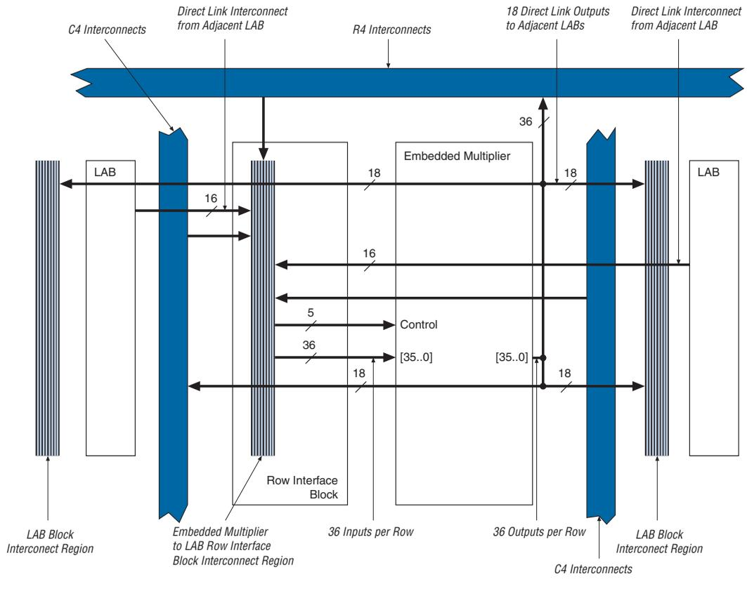
There are five dynamic control input signals that feed the embedded multiplier: `signa`, `signb`, `clk`, `clkena`, and `aclr`. `signa` and `signb` can be registered to match the data signal input path. The same `clk`, `clkena`, and `aclr` signals feed all registers within a single embedded multiplier.
