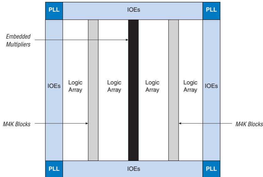
The number of M4K memory blocks, embedded multiplier blocks, PLLs, rows, and columns vary per device.
