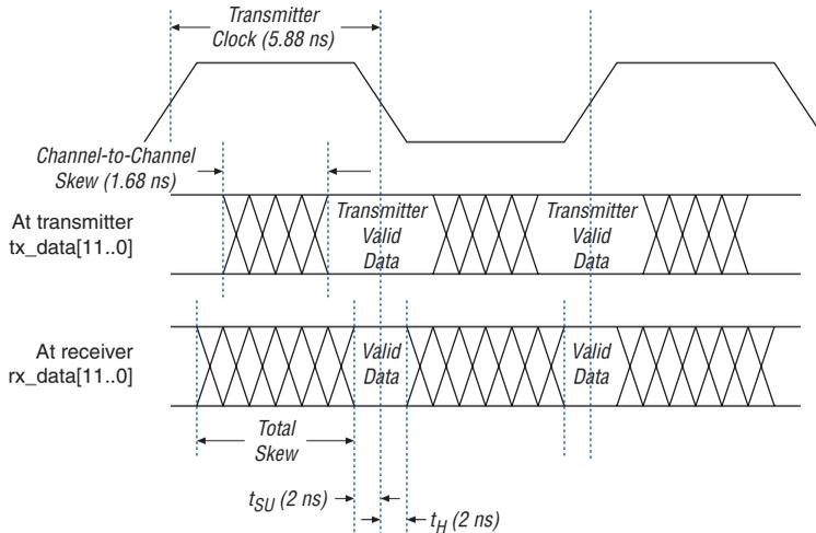
Table 5–49 shows the mini-LVDS transmitter timing budget for Cyclone II devices at 311 Mbps. Cyclone II devices cannot receive mini-LVDS data because the devices are intended for applications where they will be driving display drivers. A maximum mini-LVDS data rate of 311 Mbps is supported for Cyclone II devices using DDIO registers. Cyclone II devices support mini-LVDS only in the commercial temperature range.
