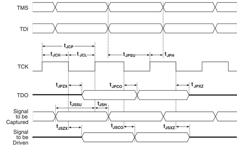
Table 5–53 shows the JTAG timing parameters and values for Cyclone II devices.
