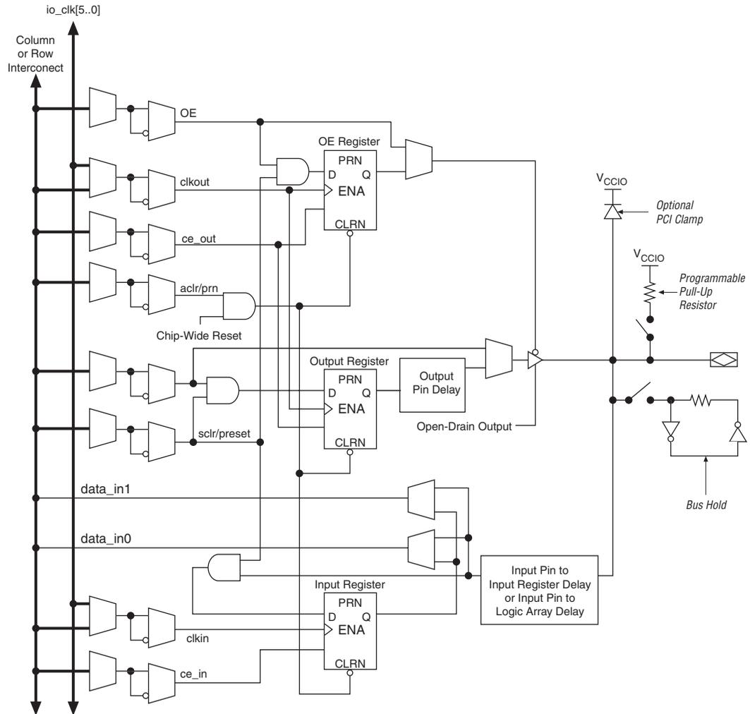
The Cyclone II device IOE includes programmable delays to ensure zero hold times, minimize setup times, or increase clock to output times.
