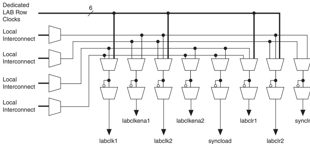
LAB-wide signals control the logic for the register's clear signal. The LE directly supports an asynchronous clear function. Each LAB supports up to two asynchronous clear signals (`labclr1` and `labclr2`).
