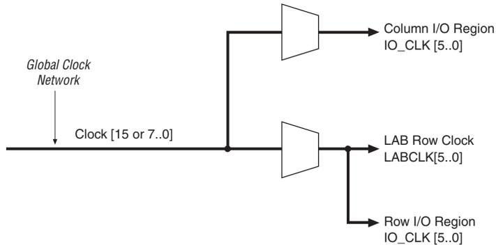
LAB row clocks can feed LEs, M4K memory blocks, and embedded multipliers. The LAB row clocks also extend to the row I/O clock regions.
