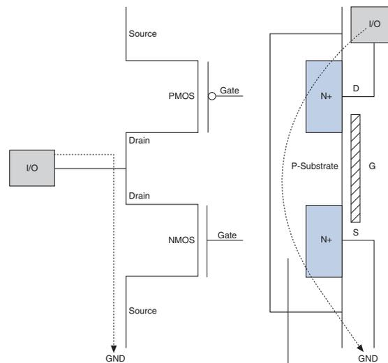
When the I/O pin receives a negative ESD zap at the pin that is less than  $-0.7\text{ V}$  ( $0.7\text{ V}$  is the voltage drop across a diode), the intrinsic P-Substrate/N+ drain diode is forward biased. Therefore, the discharge ESD current path is from GND to the I/O pin, as shown in Figure 4-4.
