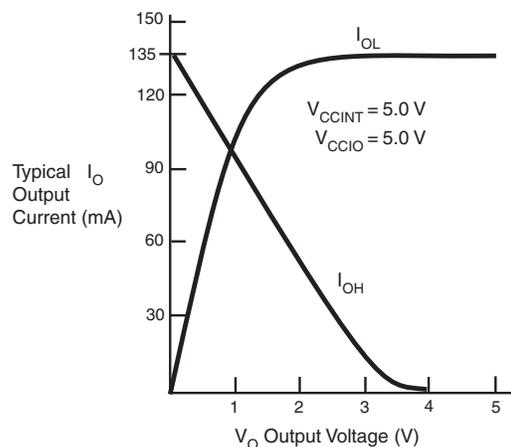
As shown in Figure 5-5,  $R_1 = 5.0 \text{ V} / 135 \text{ mA}$ .
