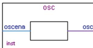
This megafunction is in the I/O folder on page 2a of the MegaWizard Plug-In Manager. On page 3 of the MAX II/MAX V Oscillator megafunction, you have an option to choose to simulate the OSC output port at its maximum or minimum frequency during the design simulation. The frequency chosen is only used as a timing parameter simulation and does not affect the real MAX V device OSC output frequency.
