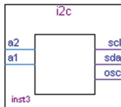
ALTUFM\_I2C megafunction is under the **Memory Compiler** folder on page 2a of the MegaWizard Plug-In Manager. On page 3, you can choose whether to implement the **Read/Write** or **Read Only** mode for the UFM. You also have an option to choose the memory size for the ALTUFM\_I2C megafunction as well as defining the four MSBs of the slave address (default 1010).
