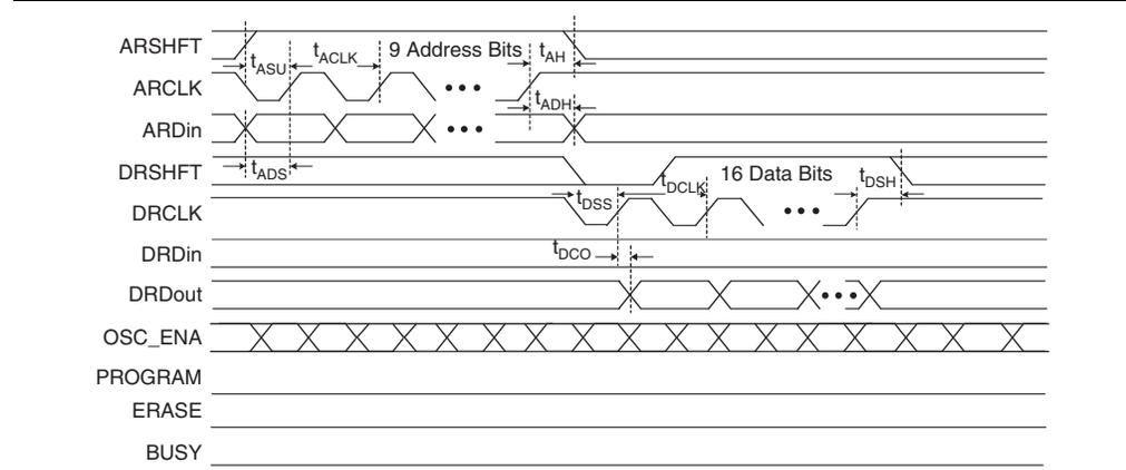
**Figure 7-6. UFM Stream Read Waveforms**
