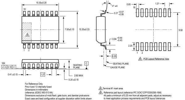
Exact case and lead configuration at supplier discretion within limits shown
