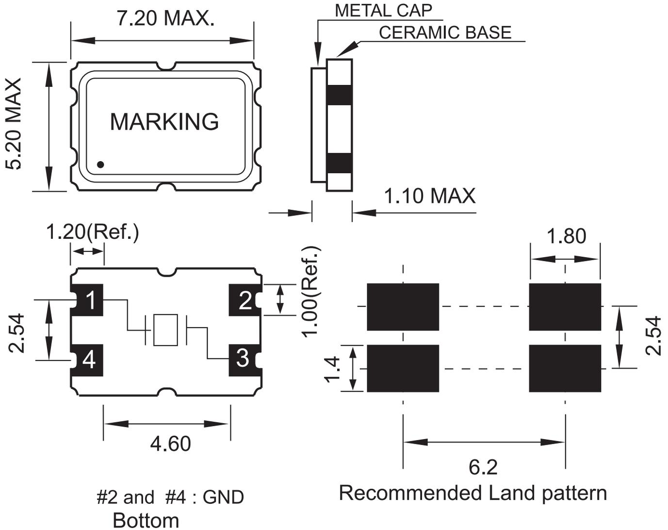
**Package is Seam Sealed Ceramic-Metal.
