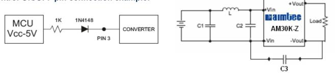
Note A: An external filter capacitor is required if the module has to meet EN61000-4-4 and EN61000-4-5. The filter capacitor Aimtec suggests: 1000uF, 100V.
