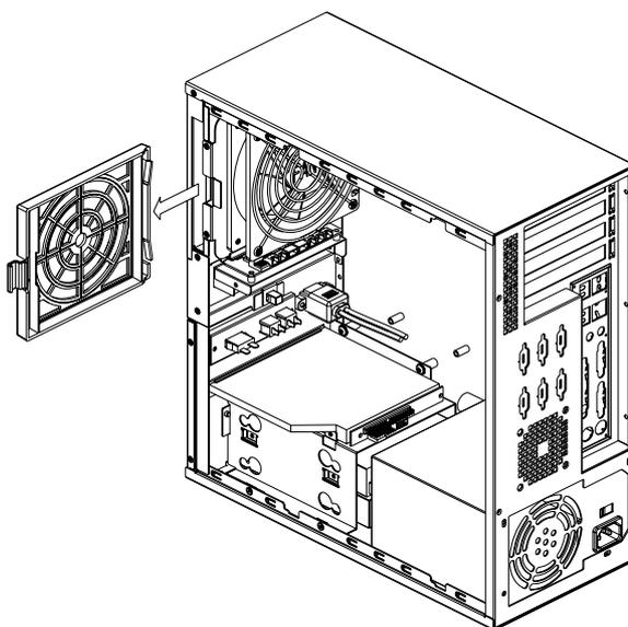
**Figure 3.6 Replacing the filters**
