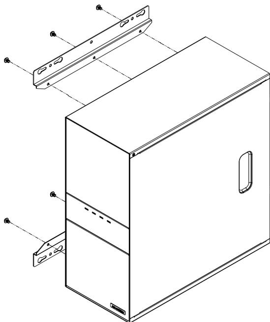
**Figure 2.7** Installing wallmount brackets
