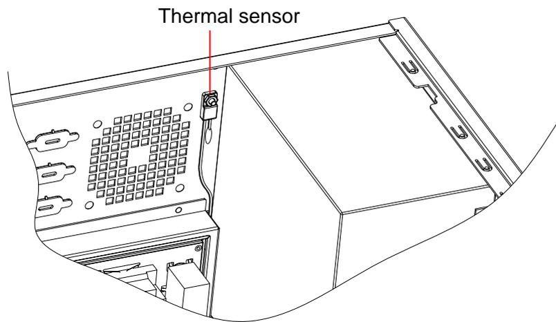
**Figure 4.2 Thermal sensor location**
