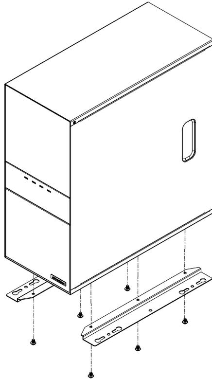
**Figure 2.6** Installing wallmount brackets
