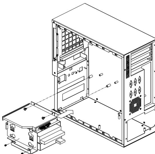
**Figure 2.5** Installing disk drive
