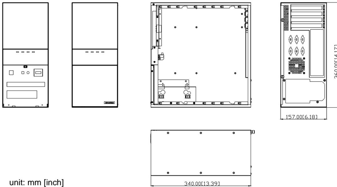
**Figure 1.1 Dimension diagram**
