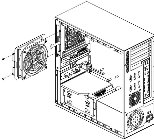
**Figure 3.4 Replacing the cooling fan**
