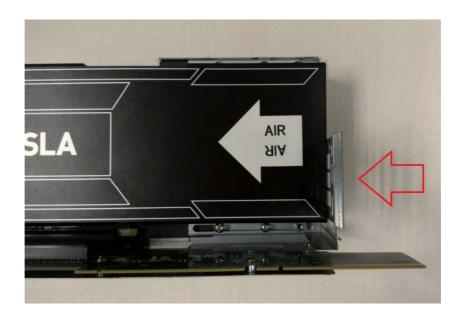
8. Screw the card holder onto the expansion card.
