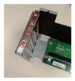
5. Install the expansion card into the card cage.
