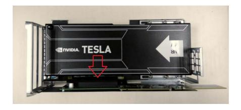
6. Screw the expansion card IO bracket onto the card cage.
