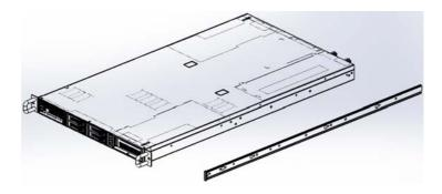
3. Attach the cabinet (outer) member to the rail. Insert the stag into the upper and lower square holes on EIA rail from the back of rail. Push the safety lock forward to secure the bracket. It is important to check if the safety lock is in unlocked position before mounting the brackets.
