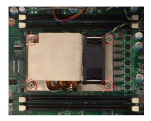
8. Repeat the procedures earlier to install the second processor and heatsink.
