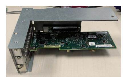
3. Install the expansion card onto the riser card.
