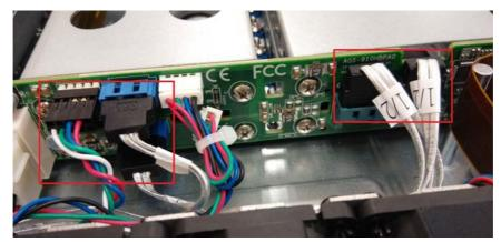
7. Install the SATA & SGPIO connector\* into HDD back plane.
