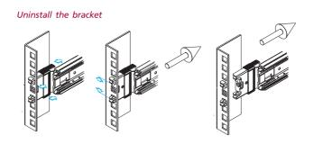
4. Mount the chassis into the cabinet. Insert the chassis (inner) member into the cabinet member as shown on the drawing. It is important to check if the ball retainer is in fully open position before install the chassis. It might cause catastrophic damage to the chassis if ball retainer is not in fully open position while mounting the chassis. While you are pushing chassis back to the cabinet, you need to release the slide from locking position by pressing the trigger down.
