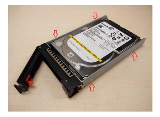
4. Re-insert the HDD tray into the chassis and press the locking lever to secure the tray.
