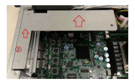
2. Screw the expansion card onto the riser card bracket.
