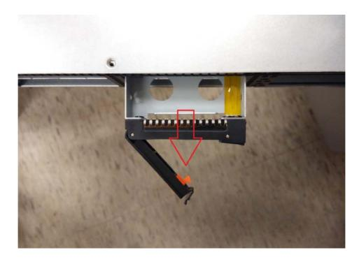
3. Place a hard drive into the drive tray, then use the screws to secure the HDD.
