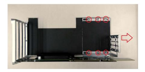
4. Unscrew the IO bracket from the card cage.
