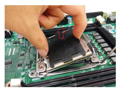
6. Close the CPU socket cover and press the lever down to secure the CPU.
