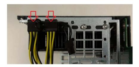
10. Put the card cage back into the chassis, and make sure the cage has no mechanical conflict with the chassis.
