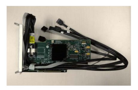
5. Install the expansion card into the chassis and secure it.
