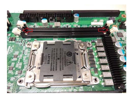
3. Align the memory module with the slot. When inserted properly, the memory slot locking levers lock automatically onto the indentations at the ends of the module.
