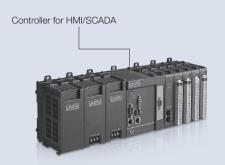
One controller focuses on I/O processing, while another controller can execute other tasks such as HMI/SCADA, database, recipe, image processing, etc. This architecture ensures system reliability since I/O processing won't be affected by other tasks.
