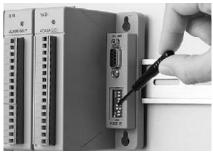
Node ID Setting 8-pin dip switch configuration
