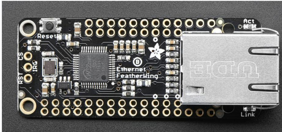
The Ethernet FeatherWing plugs into any Feather and adds hard-wired networking. To make it as cross-platform compatible as possible, we use only SPI plus one extra, configurable pin. It's not going to be gigabit (or even multi-megabit) speeds but it will work!
