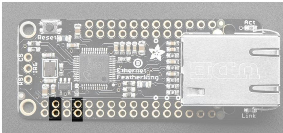
The WIZ5500 Ethernet chip (and really any ethernet chip) are fairly high current devices, requiring about 150mA whether or not actively transmitting. The chip is powered from the **3.3V** and **GND** pins indicated and does not have an internal regulator.
