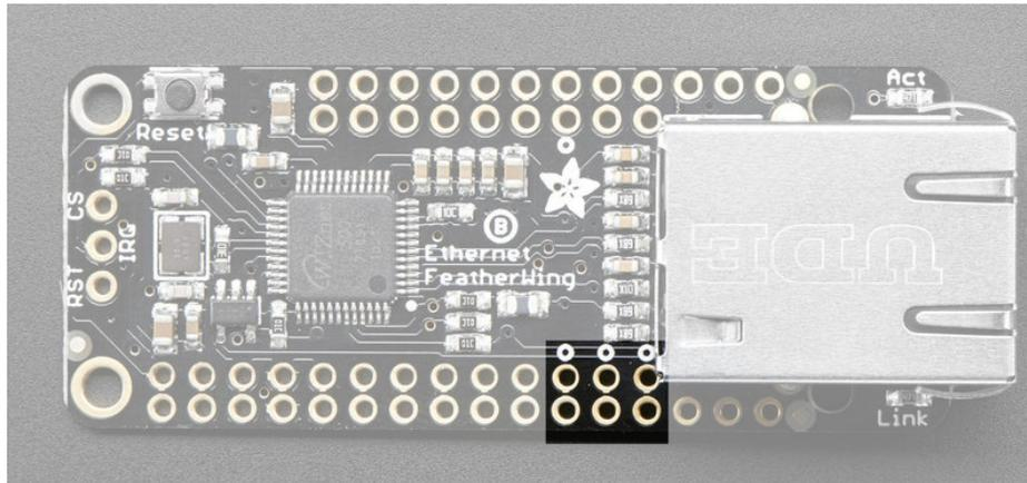
Configuration, setup, and data is received/transmitted over SPI. All Feathers have the default SPI port on the same pins, so we use **MOSI/MISO/SCK** in this location. They are 3.3V logic, 5V tolerant.
