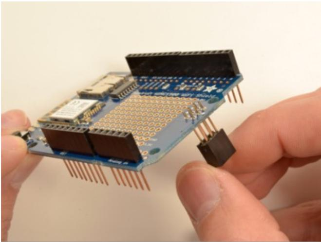
Insert the 2x3 stacking header as shown.
