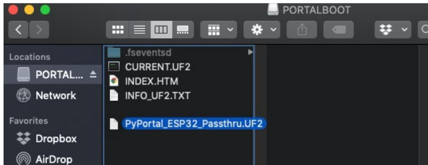
The lights should flash again, `BOOT` will disappear. Your board should re-enumerate USB and appear as a COM or Serial port on your computer. Make a note of the serial port by checking the **Device Manager** (Windows) or typing `ls /dev/cu*` or `/dev/tty*` (Mac or Linux) in a terminal.
