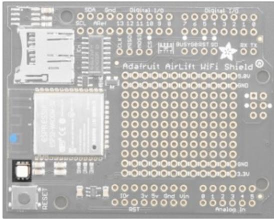
There is a small RGB LED to the left of the ESP32. These RGB LEDs are available in the Arduino and CircuitPython libraries if you'd like to PWM them for a visual alert. They're connected to the ESP32's pins 26 (**Red**), 25 (**Green**), and 27 (**Blue**).
