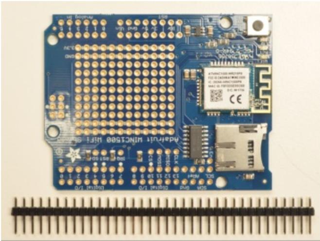
Break apart the 0.1" header into 6, 8 and/or 10-pin long pieces and slip the long ends into the headers of your Arduino.
