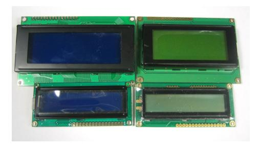
Although they display only text, they do come in many shapes: from top left we have a 20x4 with white text on blue background, a 16x4 with black text on green, 16x2 with white text on blue and a 16x1 with black text on gray.
