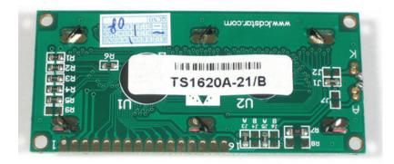
For this part of the tutorial, we'll be using LCDs with a single strip of 16 pins as shown above. There are *also* some with 2 lines of 8 pins like so:
