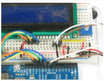
Next are the remaining 3 data lines, **DB6** (pin #13 yellow) **DB5** (pin #12 green) and **DB4** (pin #11 blue) which we connect to Arduino #11, 10 and 9.
