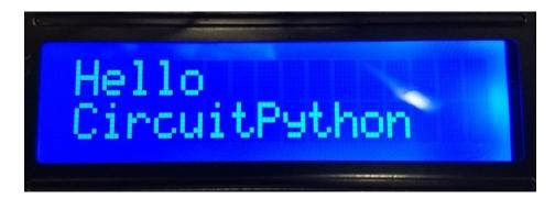
You can turn the cursor on and off using the cursor property. Set to True to turn it on and False to turn it off, for example to turn on:
