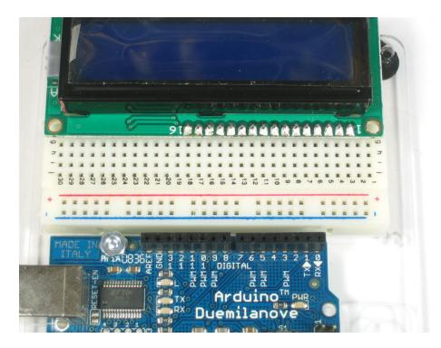
The easiest way we know of doing this is sticking the header into a breadboard and then sitting the LCD on top while soldering. this keeps it steady.
