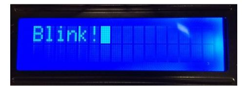
If you're using the RGB backlight display there's one extra function you can use to change the backlight color. Use the color function and provide a three-member list of red, green, blue color values, i.e. [R, G, B], that range from 0 to 100. For example to set the color to red:
