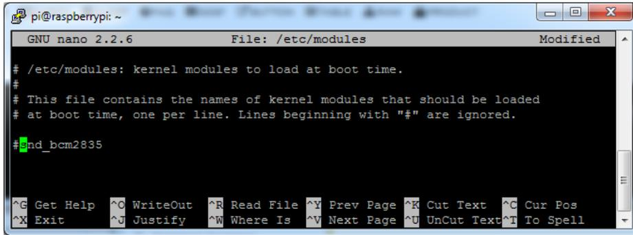
A screenshot of a terminal window on a Raspberry Pi. The window title is 'pi@raspberrypi: ~'. The terminal shows the GNU nano 2.2.6 editor editing the file '/etc/modules'. The content of the file is as follows:
