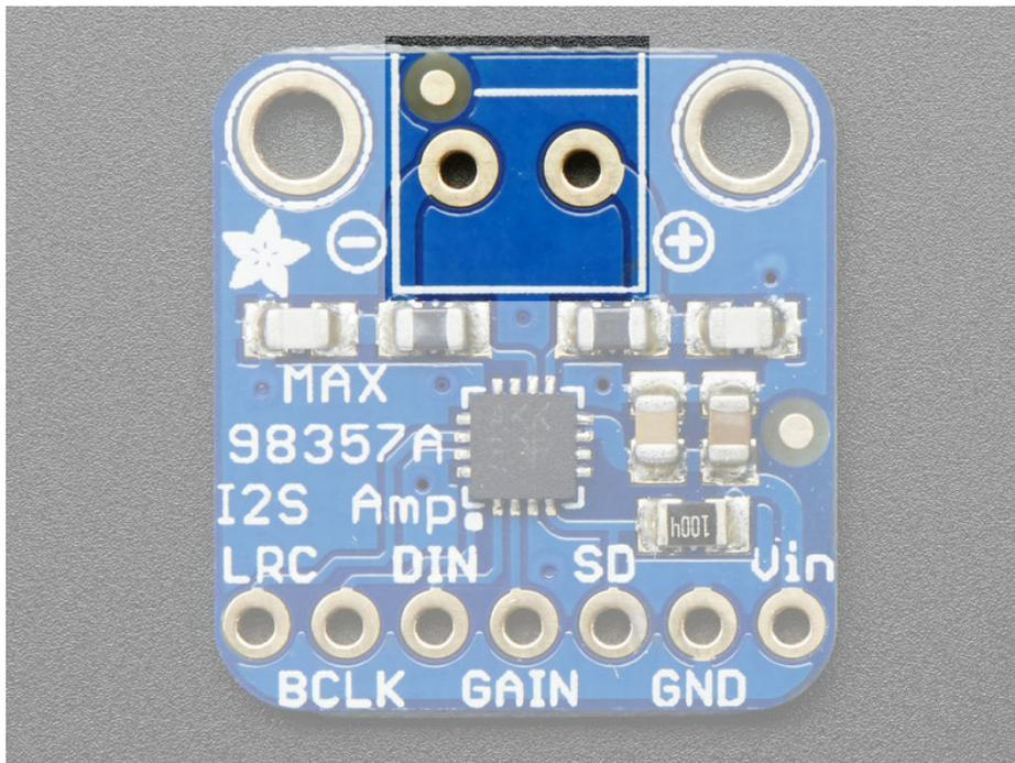
This amplifier is designed to drive moving coil loudspeakers only. Speaker impedance must be  $4\Omega$  or more. The
