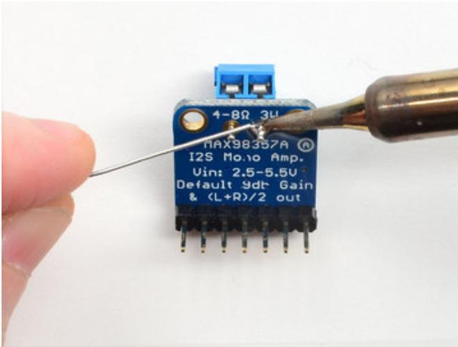
Solder in both pins with plenty of solder!
