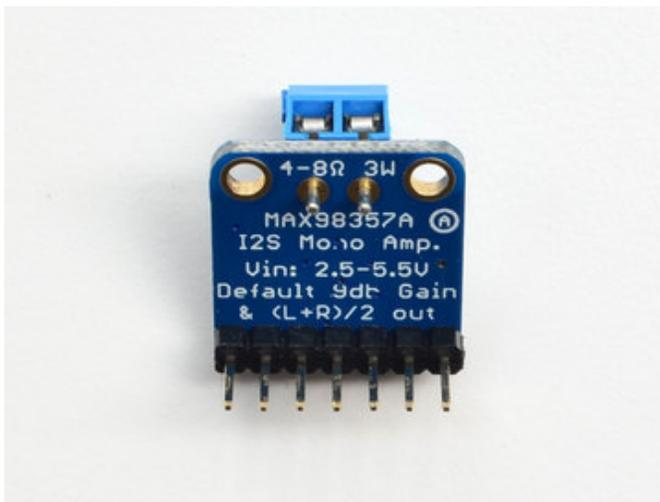
If you want to use a terminal block for connecting a speaker, place the 3.5mm terminal so the mouths point out.
