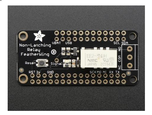
A Feather board without ambition is a Feather board without FeatherWings! These are the **Mini Relay FeatherWing.** They will give you power to control, and control over power. Put simply, you can now turn on and off lamps, fans, solenoids, and other small appliances that run on up to 250VAC or DC power using any Feather board.
