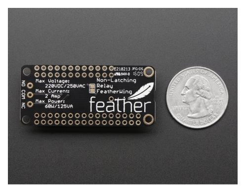
Each FeatherWing comes with a fully assembled and tested PCB, header you can use to attach to your feather. You
