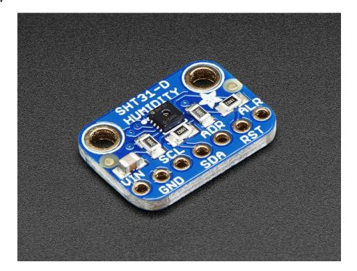
Sensirion Temperature/Humidity sensors are some of the finest & highest-accuracy devices you can get. And, *finally* we have some that have a true I2C interface for easy reading. The **SHT31-D** sensor has an excellent  $\pm 2\%$  relative humidity and  $\pm 0.3$ °C accuracy for most uses.
