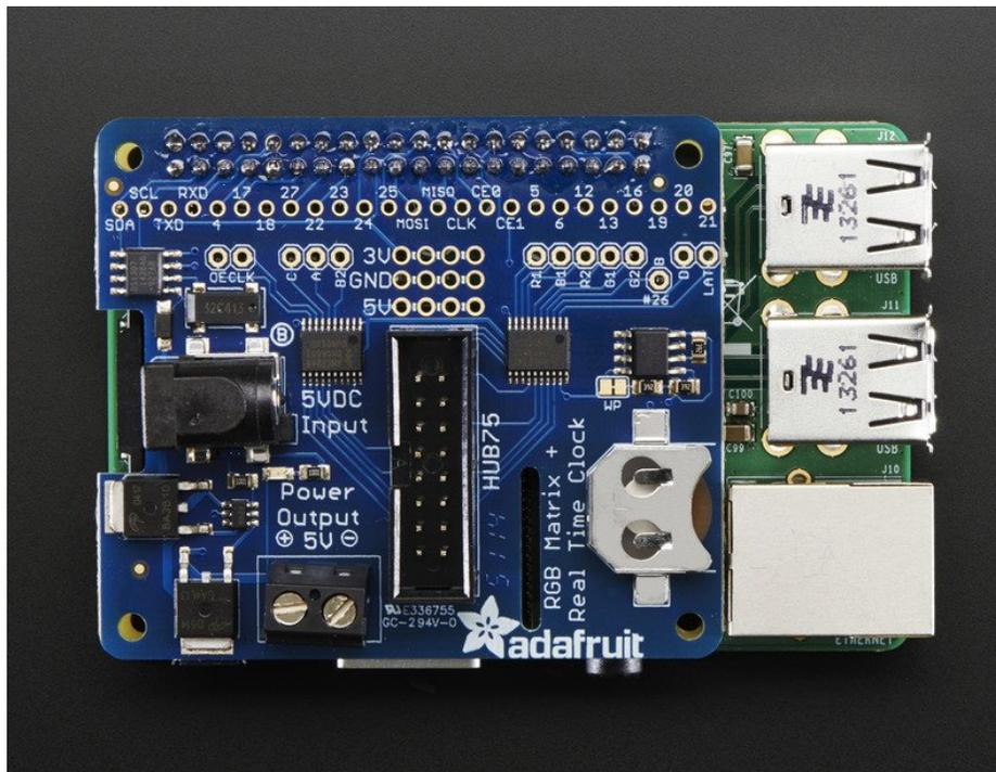
Each order comes with a HAT PCB with all surface mount parts assembled, a 2x20 female socket connector, a 2 pin terminal block, and a 2x8 IDC socket connector. [A CR1220 coin cell is not included to make air shipping easier, please order one separately \(https://adafru.it/em8\)](https://adafru.it/em8) if you do not have one and would like to use the real time clock.
