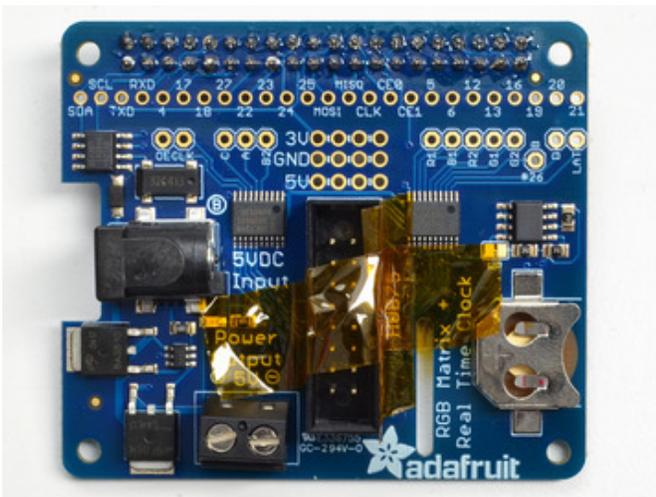
Use some tape to hold the IDC connector in place
