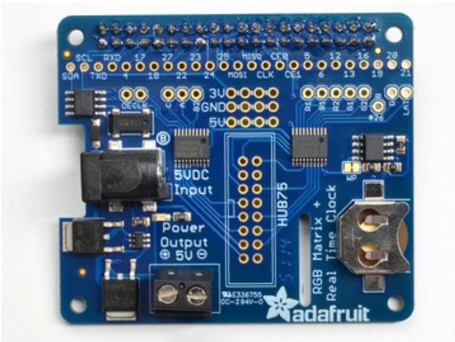
Next up we will attach the 2x8 IDC header. Unlike the 2x20 header, **this connector has a direction!**
