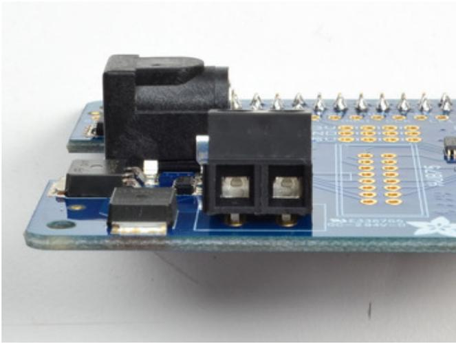
Place the 2 pin terminal block first, make sure the two 'mouths' are facing outwards
