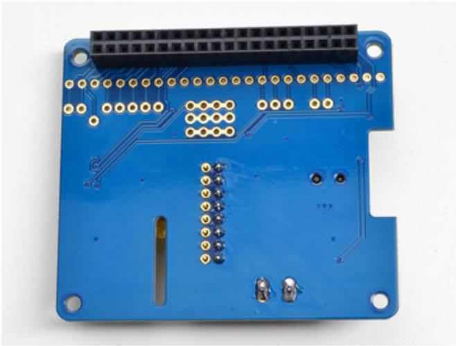
Check your work! Make sure all the solder points are clean and not shorted or cracked or dull
