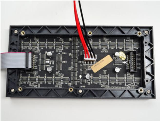
IDC goes into the INPUT side (look for any arrows, arrows point from INPUT side to OUTPUT)
