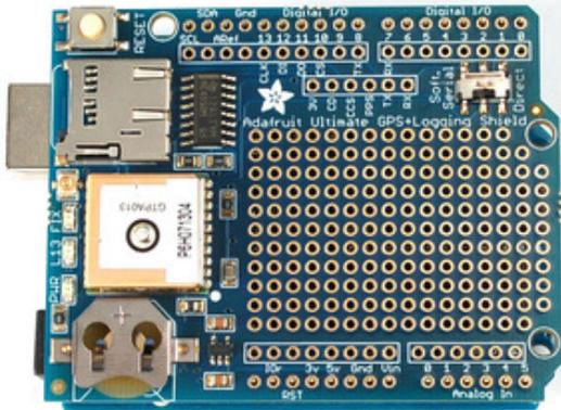
Place the shield on top so the short ends stick out thru the PCB, solder all the pins
