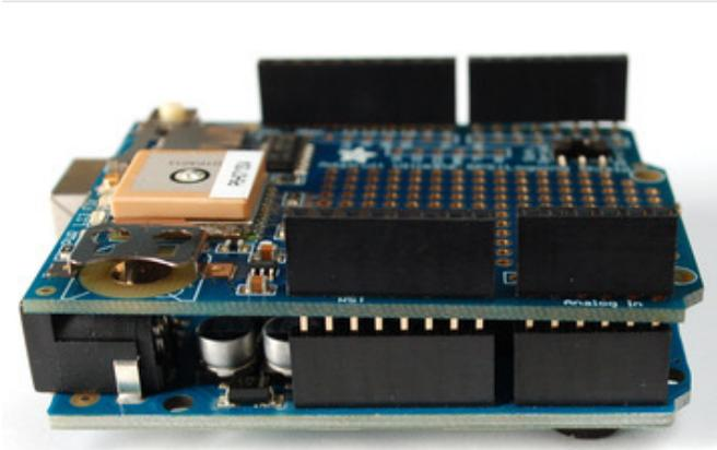
Fit the long pins through the pads until they slot into the Arduino. Depending on which version/type of Arduino you may need to use 2 x 8pin and 2 x 6pin *or* 1 x 10pin, 2 x 8pin and 1 x 6pin.
