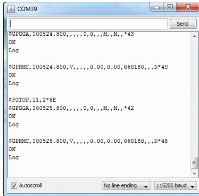
If the SD card was initialized OK, it will read a sentence from the GPS, check the checksum and if its a proper sentence, and then log it.
