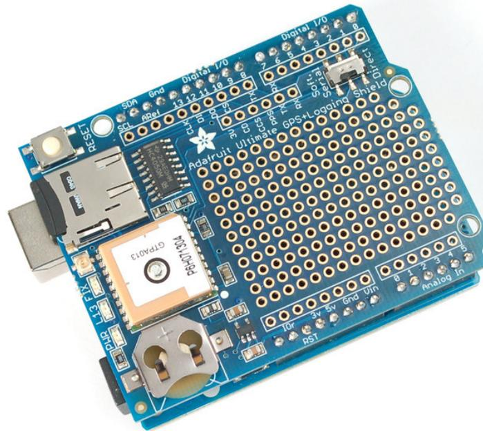
Brand new and better than ever, we've replaced our Adafruit GPS shield kit with this assembled shield that comes with an Ultimate GPS module. This GPS shield works great with either UNO or Leonardo Arduinos and is designed to log data to an SD card. Or you can leave the SD card out and use the GPS for a geocaching project, or maybe a music player that changes tunes depending on where you are in the city.
