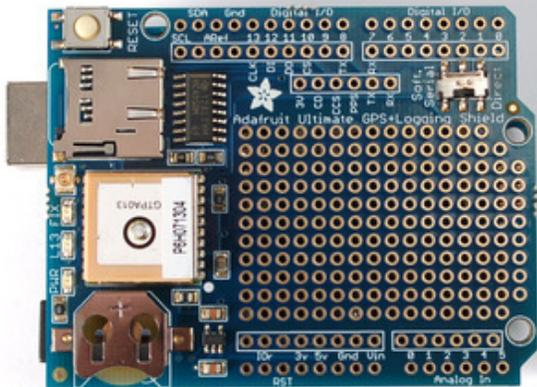
If you want to go with stacking headers, place the the shield PCB on top of the Arduino
