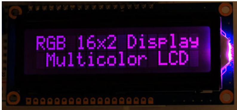
You can also use 16x2 LCDs that are the same size that do not have an RGB backlight, or have no backlight at all.
