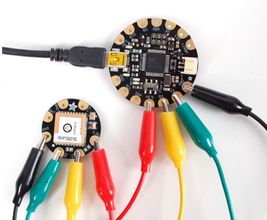
Use alligator clips to connect Flora's 3.3V pad to the 3.3V pad on the GPS. Likewise connect RX to TX and TX to RX, then finally GND to GND.
