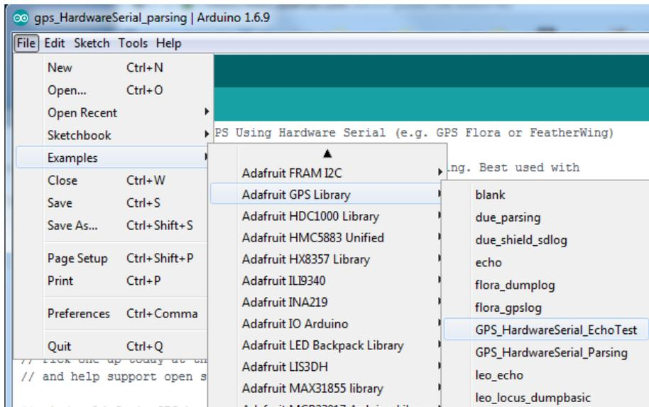
Wire up the GPS module according to the hookup. [Check your board and serial port settings \(https://adafru.it/aRS\)](https://adafru.it/aRS) and upload this sketch to your Flora using the Upload button in the IDE. Open up the **Serial Monitor**.
