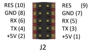
J2 Pinout (Programming Header)
