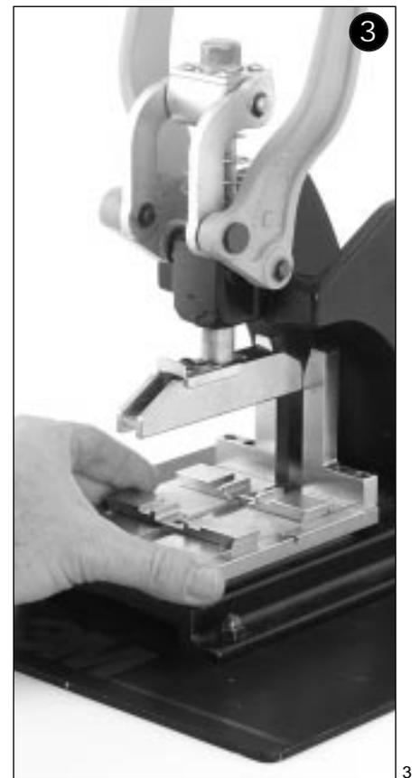
Place the 10982-4 height gauge on the base plate of the press (locator plate removed). Bring the handle down fully and adjust the shaft to touch the gauge. Raise the handle, remove the gauge then turn the adjustment screw one quarter turn (90 degrees) clockwise.
